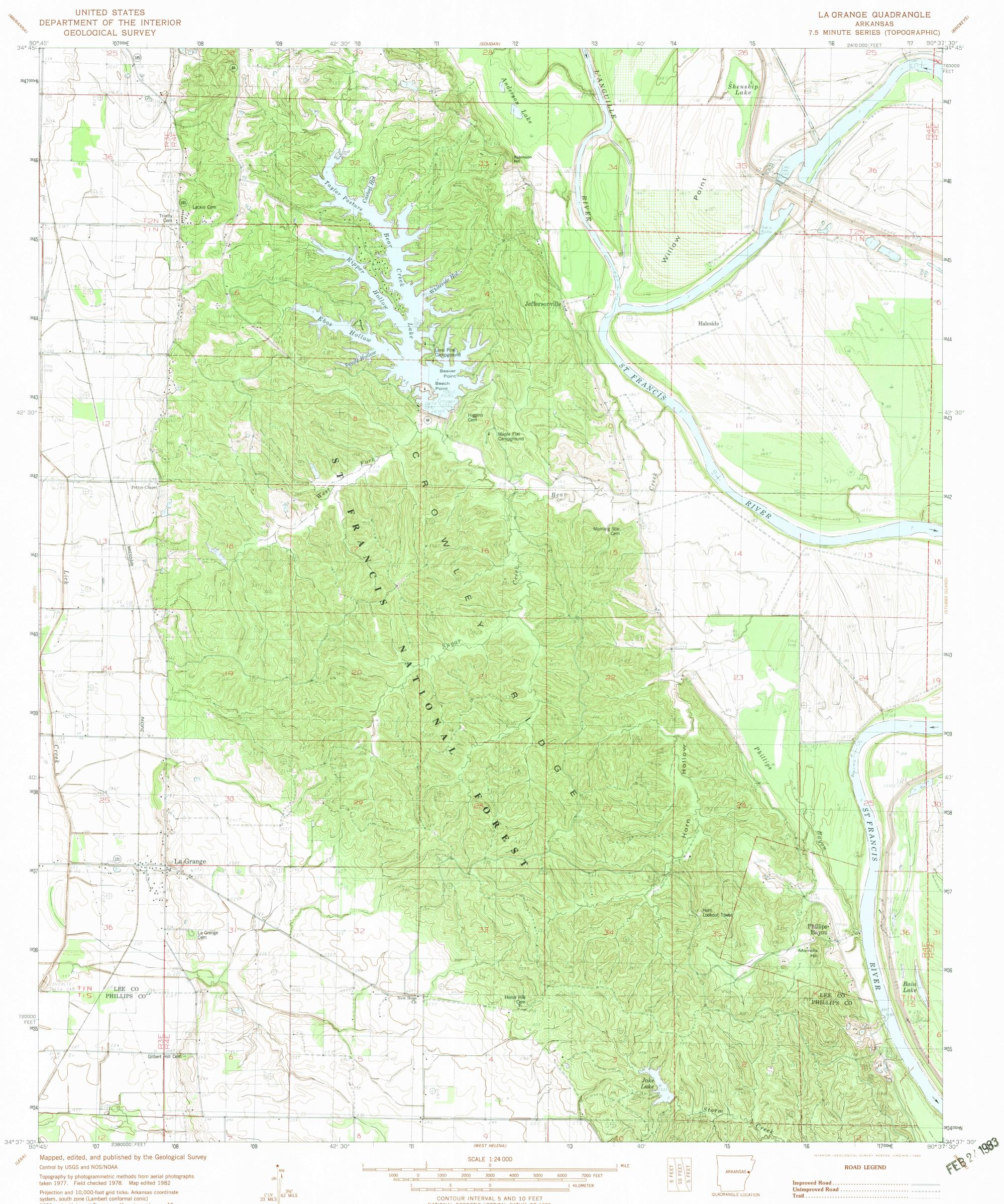
system, south zone (Lambert conformal conic) 1000-meter Universal Transverse Mercator grid, zone 15 1927 North American Datum To place on the predicted North American Datum 1983 move the projection lines 8 meters south and 10 meters east as shown by dashed corner ticks
