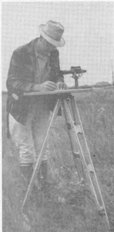
Topographic mapping with plane table.
