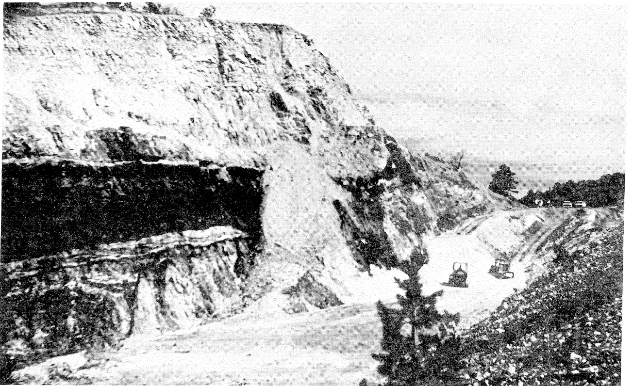
Figure 4. Malvern Minerals Company novacite (tripoli) mine in Garland County, Arkansas. The Arkansas Novaculite is inverted with the white tripolitic novaculite of the Upper Division at the base, the dense novaculite of the Lower Division at the top, and the black carbonaceous shale of the Middle Division occurring between them. Photograph by John David McFarland, III, Arkansas Geological Commission.
